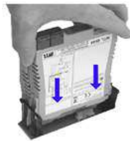
Figure 240: Mounting a module onto an IOTA
